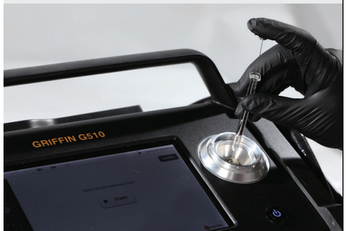
Syringe injection performed on Griffin G510
