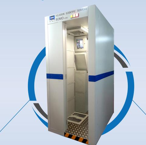
It includes 26 plastic scintillators + ZnS designed to measure alpha and beta particles which work autonomously and independently, allowing to perform simultaneous measurements with different alarm levels.
