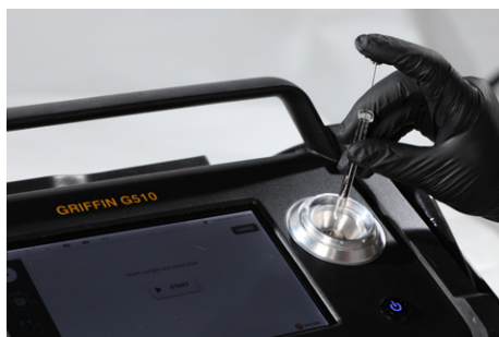
Fig 4 Direct syringe injection performed on Griffin G510
