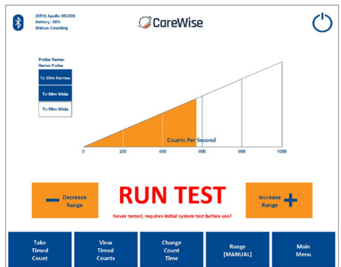
Figure 30 – Main Counts screen showing indication for running a System Test if a new OmniProbe or Apollo handset is selected and has never had a System Test before
