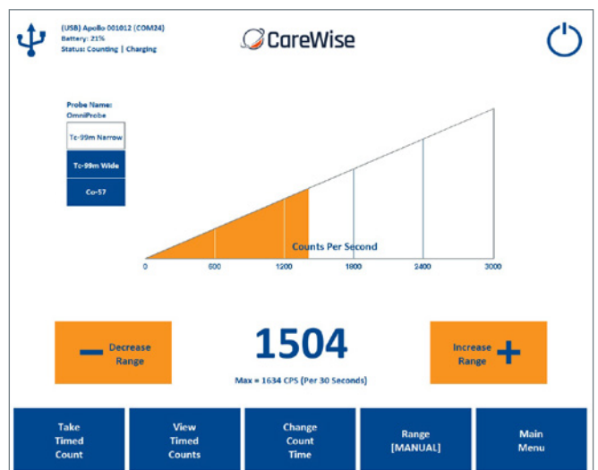
Figure 21b – Main Count Screen showing the USB icon for the active USB wired Apollo handset mode of operation
