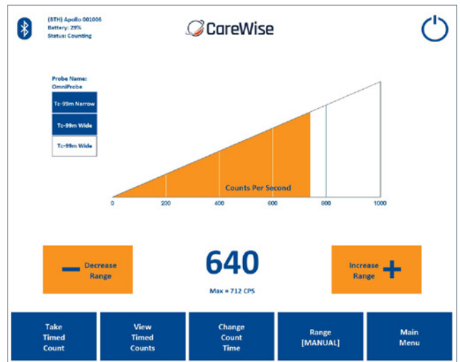
Figure 29 – Main Counts Screen showing Apollo handset has become active again after a Sleep period
