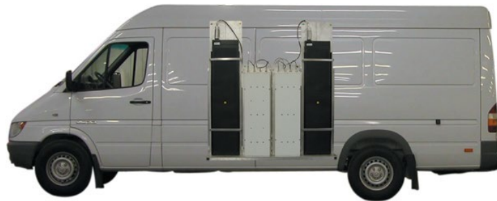
Cut-away view of the TSA MD134 mounted in a van for mobile screening. (Van is not included.)
