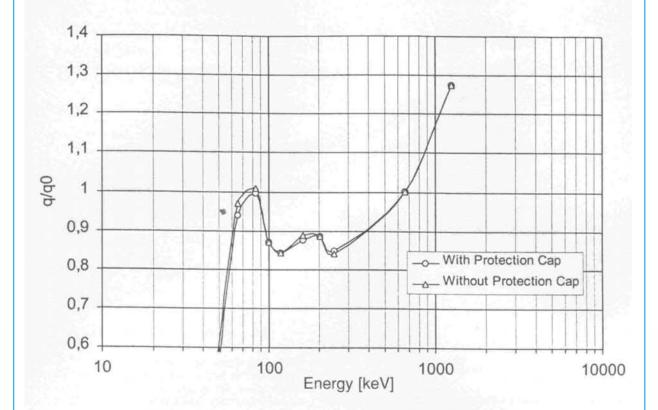
Energy dependence referred to H<sub>x</sub>, normalised to Cs-137, high range detector:
