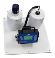
The GM/Nal(Tl) with gamma spectroscopy option would be selected if the relative background is high and windowing of the isotope is required, or the system will be used for a range of different therapy isotopes (we offer the FLIR scintiSPEC system for this).
