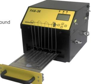
The PAB-3R low background counter allows you to measure  $\alpha$  and  $\beta$  contamination from a surface. The wide area smear tests are controlled and sorted according to the radiological thresholds and preset uncertainty.
