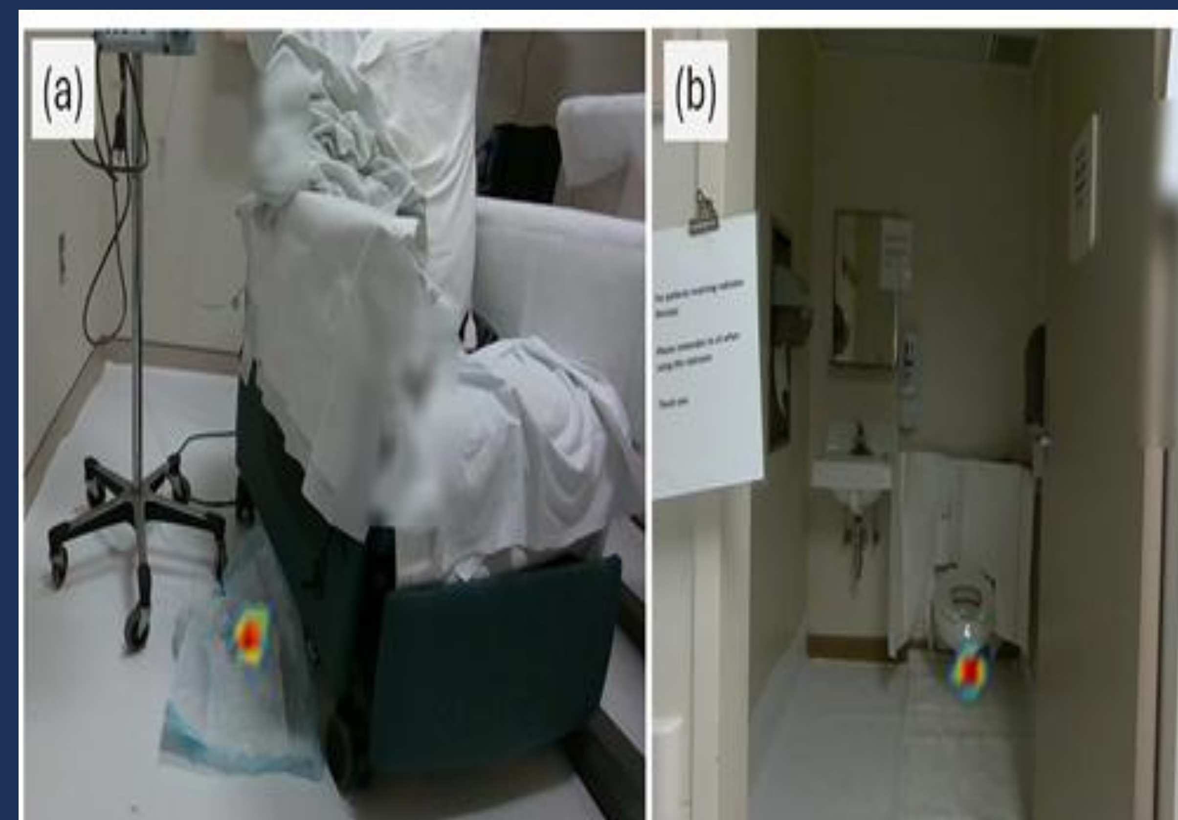
Figure 3: RISM images acquire in (a) patient treatment bay and (b) patient bathroom showing areas of contamination after Lu-177 treatment.
