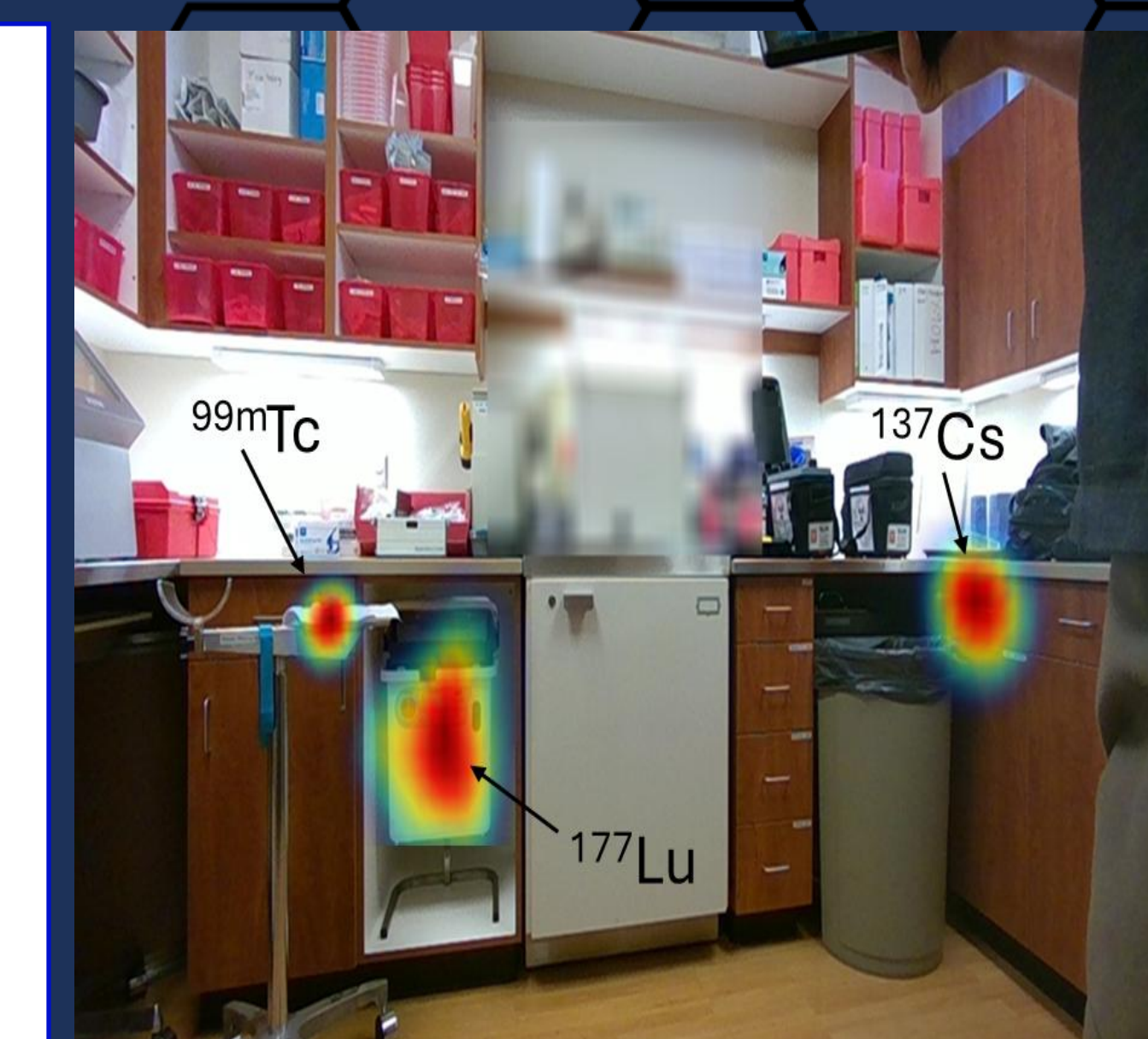
Figure 2. RISM image of location of three deliberate contamination sources (labeled) in a hot lab.
