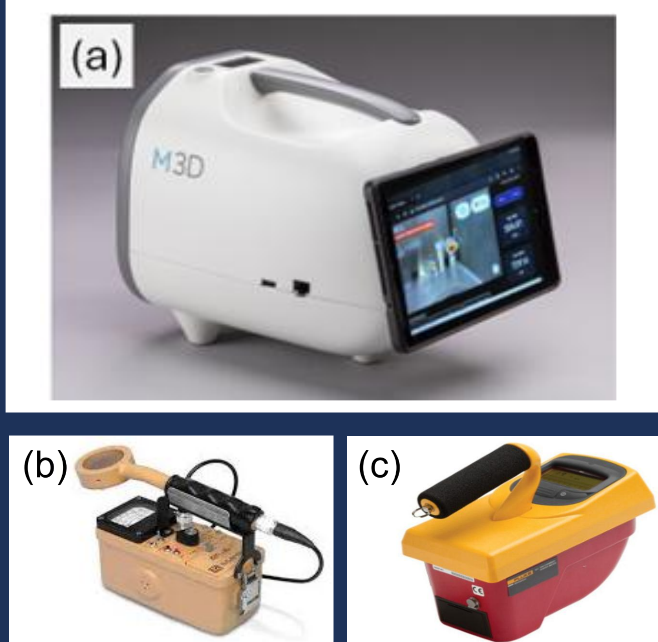
Figure 1: (a) The RAVIN RISM, (b) pancake GM counter, and (c) pressurized ion chamber.
