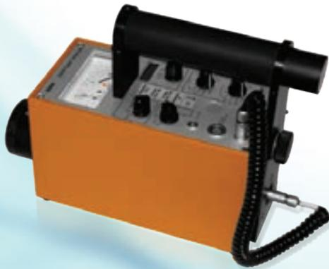
Automess highly sensitive instrument, with a large tissue equivalent scintillation probe.
