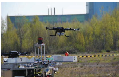
Drone landing on a platform and equipped with a SPIR-Explorer detector.
