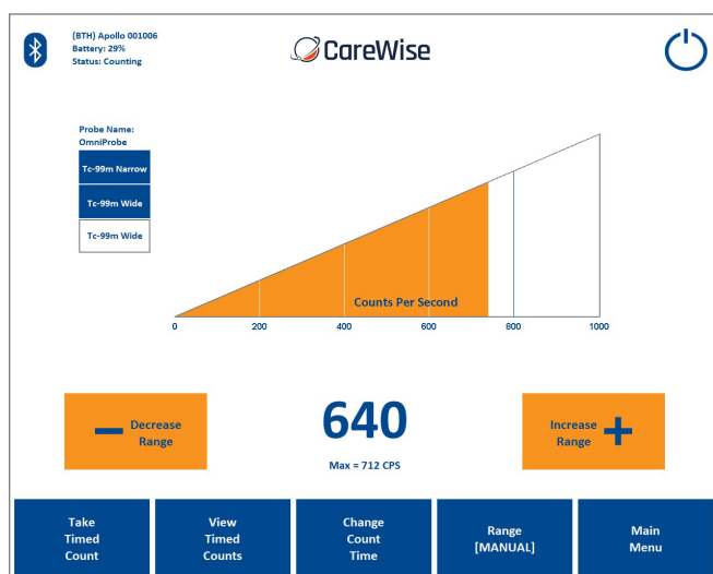
Figure 29 – Main Counts Screen showing Apollo handset has become active again after a Sleep period.
