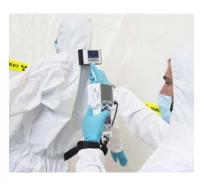
Due to its ergonomic probes, the SaphyRAD is adapted to nuclear workplace clearance control. The mobile pedestal allows the installation of mobile checkpoints.
