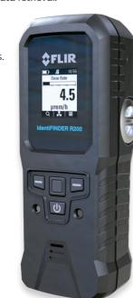
in a pager-sized device, the R300 virtually eliminates the false alarms and false positives that are so common to personal radiation detectors.
