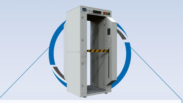
It has 8 large-area plastic scintillation detectors distributed over walls, floor and ceiling, creating 8 sensitive areas (1 foot, 2 legs, 4 torso and 1 head) that work autonomously and independently, allowing simultaneous measurements with different levels of alarm.
