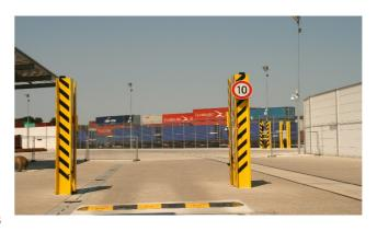
The SaphyGate G Portal detects very low radioactive sources, even when they are hidden in high density loading. This type of system has been initially designed to address issues in the nuclear industry and research, but it is now a critical building block to prevent the risks related to the use and movement of radioactive sources.
