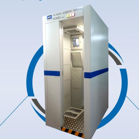
It includes 21 solid detectors (without gas) distributed as: 14 + 1 plastic scintillation detectors designed to measure beta particles and 6 plastic scintillation detectors designed to measure gamma radiation, which work autonomously and independently, allowing to perform simultaneous measurements with different alarm levels.
