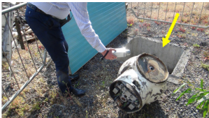
Figure 16. An abandoned radiotherapy head.
