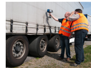
Figure 9. Examining cargo with the FLIR R500, a digital hand-held gamma radionuclide identification device (RIID).
