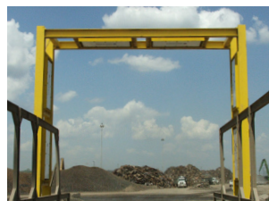
Figure 10. A portal monitor from Nucsaf, installed at a scrapyard.
