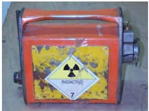
Figure 20. A gammagraphy device.
