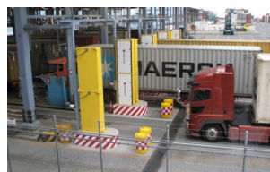
Figure 11. A portal monitor installed by Nucsaf at a dockside freight terminal.
