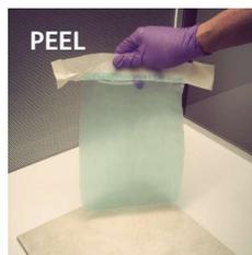
DeconGel 1101 is the 'work-horse' of the family of products highly efficient for porous surfaces. The 1120 is the 'sprayable' version of the 1101. While the sprayable feature can be an advantage, the fact that it contains more water may delay the drying time if conditions are cool and damp.
