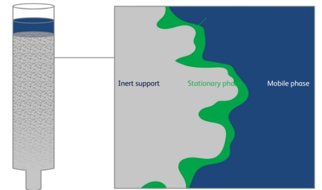
Extraction chromatography resin structure. The stationary phase contains liquid extractant compound specific to the target radionuclide.
