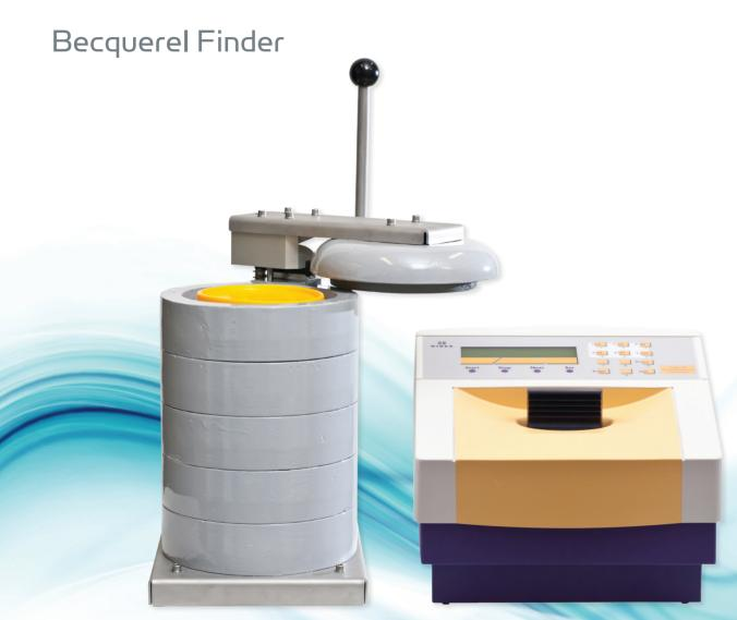
Triathler Becquerel Finder is optimized for detection of radioactive isotopes in the event of a nuclear emergency in food. The instrument is equipped with an external NaI detector with an enlarged lead shield, which facilitates the use of Marinelli beakers with total sample volume of up to 1L. This enables rapid detection of I-131, Cs-134 and Cs-137 in foodstuff, water and milk.
