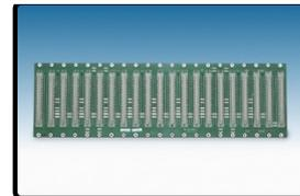
The 3U WIENER VME-J2 backplane fully complies with ANSI/VITA 1-1994 and IEEE-1014-1987 specifications. It is designed as a 4-layer board in strip-line technology. WIENER J2 VME backplanes are available with 5, 7, 9, 10, 15 or 21 (full size) slots.
