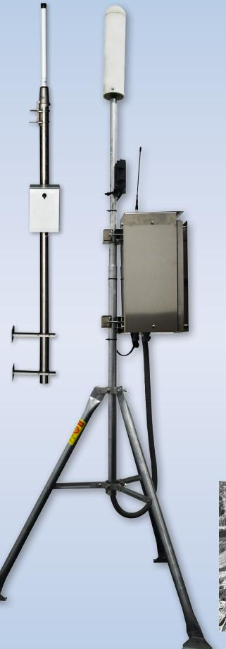
The BS/MS communication is made through a radio link in the 400 MHz band (another frequencies upon request). The standard power used is 1 W in the uplink (MS to BS) and downlink (BS to MS). The communication range depends heavily in the antenna placement and local propagation conditions but it can extend easily to several kilometers.
