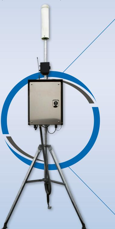
Each MS is equipped with a radioactive detector that measures the radiation levels in the air, recording the results in their internal memory. The BS can retrieve the readings interrogating each MS through the bidirectional wireless link.
