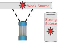
When imaging a weak source in the presence of a strong source, the H100 sees ony the strong source, but the P100 can see the weak source because of the P100's collimator.
