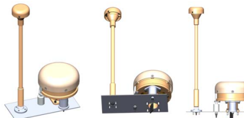
Figure 4. Top, Bottom and Side Views of the Remote Detector and Collector Sampling Stacks
