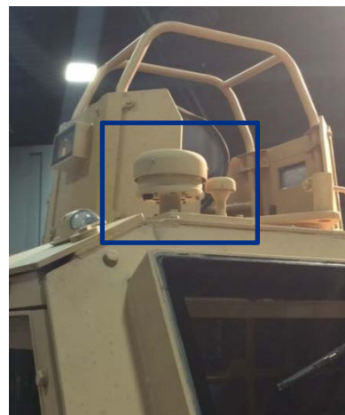
Figure 1 – Fido B2 Integrated in Military Vehicle Collector Stack (Left); Detector Stack (Right)
