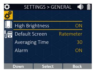
The **General Settings** screen allows the screen brightness to be changed, along with the default user screen, integrated measurement averaging time and count rate alarm level.
