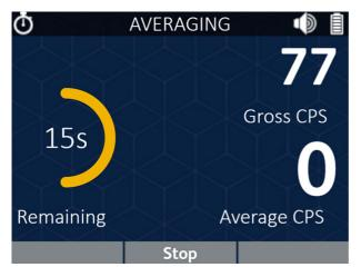
If the **Averaging** setting has been selected, the screen will change to the AVERAGING screen and allow a settable integrated count measurement to be taken.
