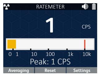
This screen is the default display of the device. The device will return to this screen when powering on. By default, it shows the current Counts Per Second (CPS) detected in the centre of the screen. The maximum (Peak) value detected during the current usage period are displayed along the bottom of the screen. These will be reset when the screen is changed or the unit is restarted.
